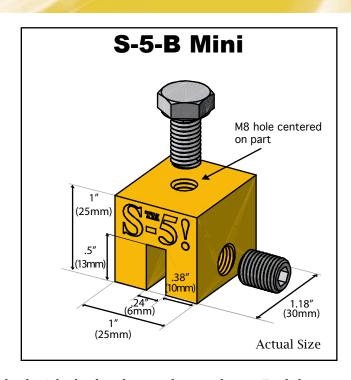
T he S-5-B and S-5-B Mini clamps are each furnished with the hardware shown above. Each box also includes a screw gun bit tip. All included hardware is stainless steel. Please visit www.S-5.com for more information including CAD details and specifications.
