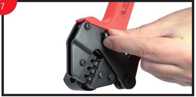
If jam occurs slightly compress handle while using fingers to rotate release clock wise.
