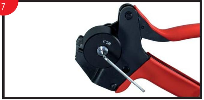
Loosen the fixing screw for changing the locator, using Allen key (2.5 mm).
