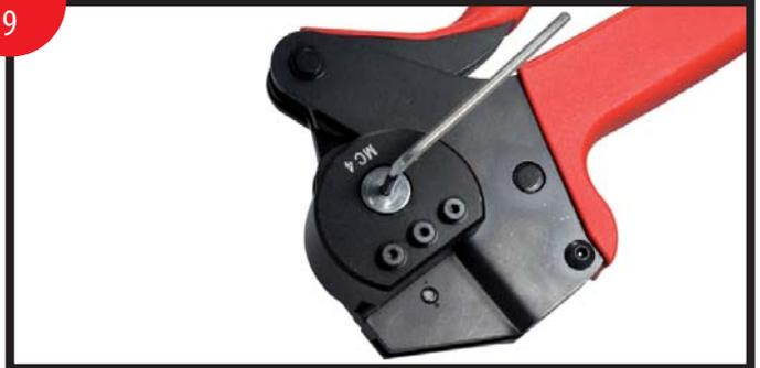
Loosen the fixing screw for changing the locator, using Allen key provided.
