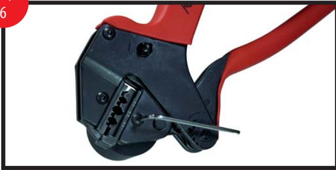
Loosen the fixing screw to change crimping dies, using Allen key (2.5 mm).
