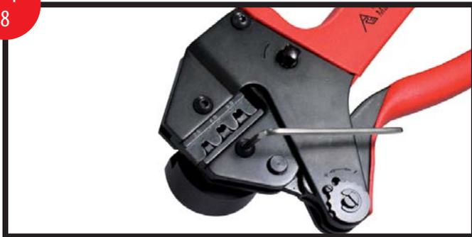
Loosen the fixing screw to change crimping dies, using Allen key provided.
