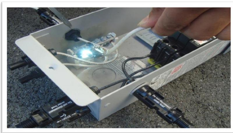
If you experience nuisance tripping you can raise the sensitivity one digit at a time. Follow the instructions below to make adjustments or disable Arc fault. As a last resort, you may disable Arc fault if your system cannot work with the arc fault detector.
