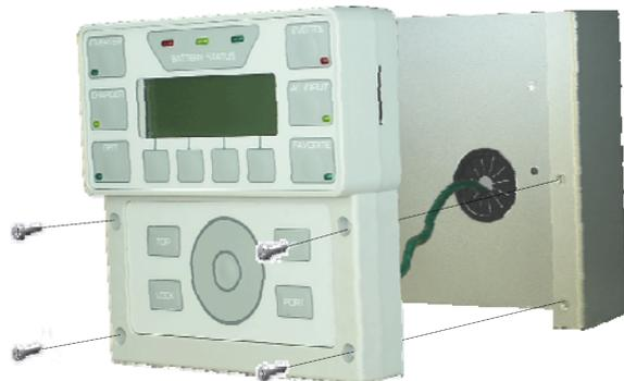
The MATE3 and bracket are now attached to the mounting surface and ready to be used.
