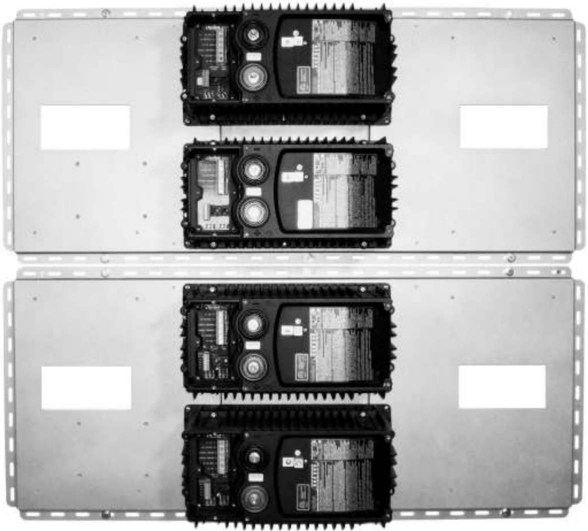
Figure 5: Four FXs installed on FW-MPs
