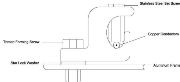
PV module grounding with lay in lug (  $\phi$  4mm grounding holes)
