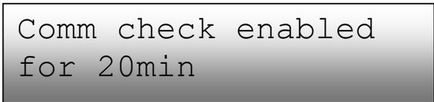
The Envoy begins a 20 minute communication check to assess the signal strength between the Envoy and the devices deployed at your site.
