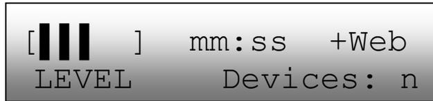
The "LEVEL" indicator in the LCD window may display any number of bars from zero to five. You can assume that the communication check is progressing normally and that signal strength is acceptable if two to five bars are displayed. If fewer than two bars are displayed, you may want to try the following options:
