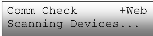
3. When the Envoy begins detecting devices (microinverters), the display reads:
