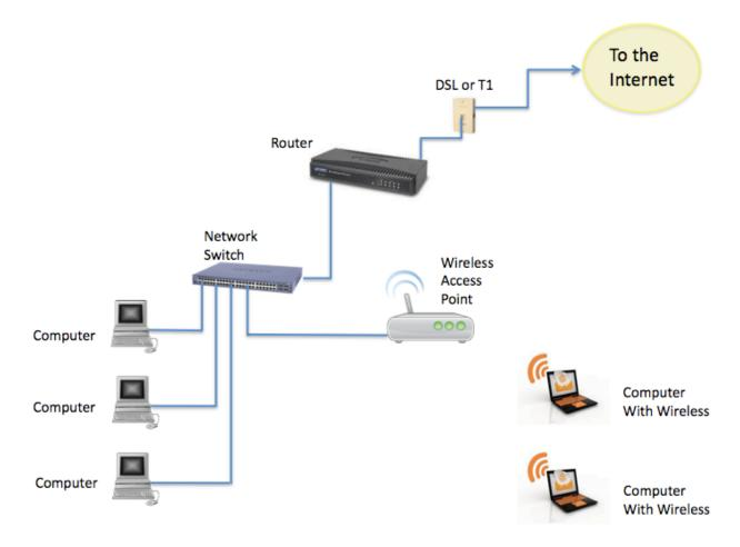
The computers are connected to the Network Switch via standard Ethernet cables. The computers with wireless (WiFi) capability access the LAN via a separate Wireless Access Point, which itself is connected to the Network Switch.
