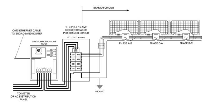
Note that there is a reference to the LAN/Ethernet cable coming into the LCF enclosure, which then plugs into the Envoy's Ethernet port. The other end of that Ethernet cable connects to an Ethernet switch or router in a network infrastructure, which ultimately leads to an Internet connection.
