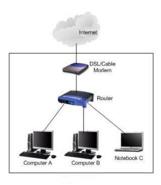
The WAN (Wide Area Network) portion is what is on the "outside" of the local network. In the diagram above, that would encompass the "WAN" port of the Router and the DSL/Cable Modem. The WAN is the upstream connection to the Internet.
