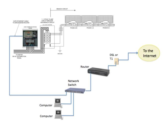
Note that the Envoy is mounted inside of the LCF enclosure, but still needs a standard Ethernet cable to an upstream Internet connection.
