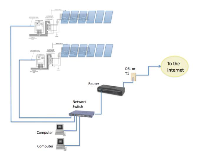
This model can scale as large as you need. For another collection of fewer than 180 microinverters, add another LCF with built-in Envoy to build discrete groups (LCF+Envoy+Microinverters) each in their own communications domain. Using the filtering mechanism of the LCF, the power line communications from one communications domain is isolated and separated from any others.
