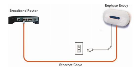
The Envoy, in this sense, acts just as another computer in the house or business, connecting through a standard Ethernet LAN cable and using standard TCP/IP protocols.
