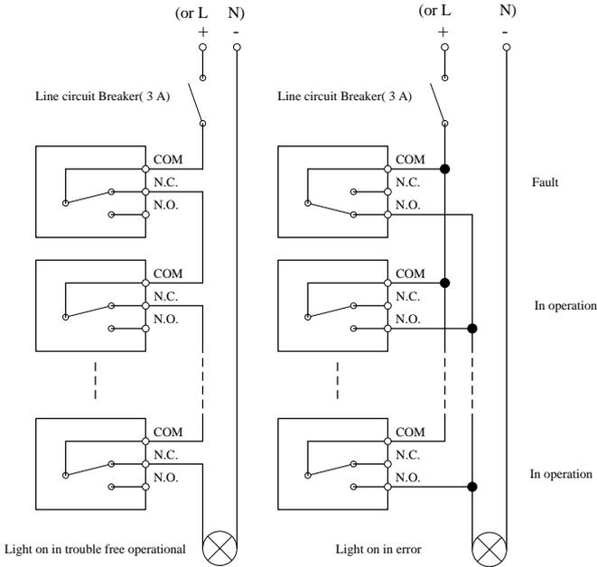
**Figure 2.35 - Dry Contact Communication Schematic Diagram**
