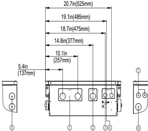
**Figure 2.17 - External Connection Ports**
