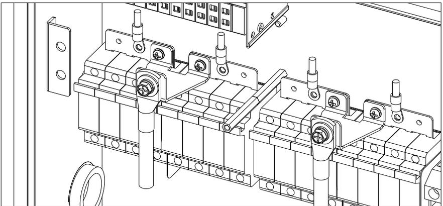
Figure 8.2 – Fuse Bypass Single Input (Combined MPPT)
