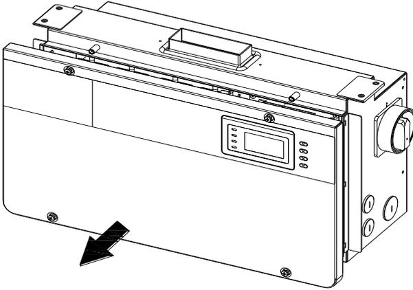
**Figure 2.15 – Removing the Wiring Box Cover**
