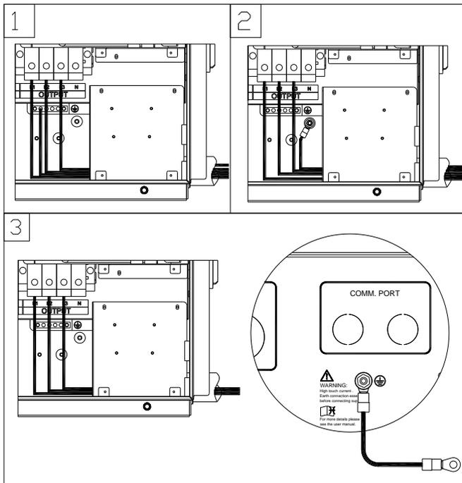
**Figure 2.29(b) - AC Output and Ground Cable Connections**
