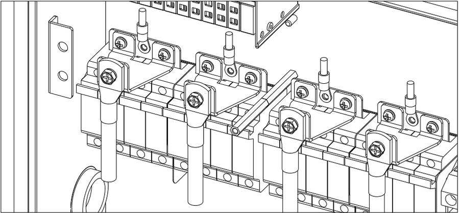
Figure 8.1 – Fuse Bypass Two Inputs (Two Independent MPPTs)
