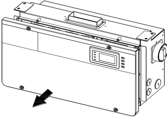
**Figure 2.28 - Remove the Wiring Box Cover**
