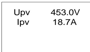
**Figure 4.9 - Operation Information Indication (PV Parallel Mode)**
