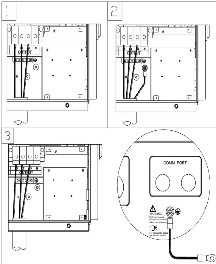
Figure 2.29(a) - AC Output and Ground Cable Connections
