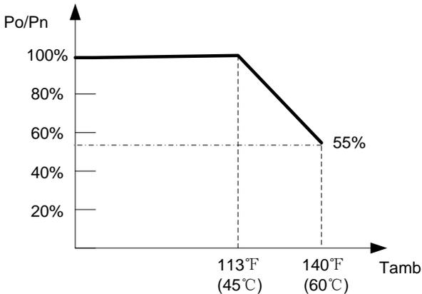
**Figure 7.2 - PVI 36TL Derating Curve with High Temperature**
