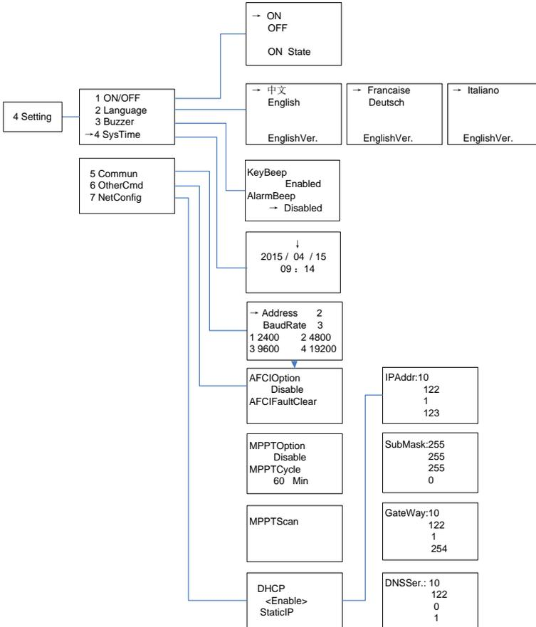
Figure 4.12 - System Setup Menu and Submenu
