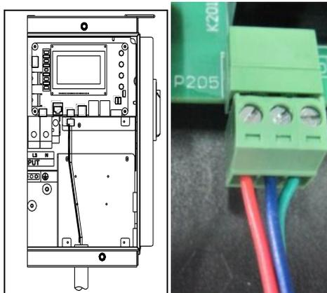
**Figure 2.38 - Dry Contact Communication Cable Connection**
