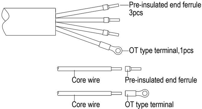
**Figure 2.31 - AC Output and Ground Cable Set Up**
