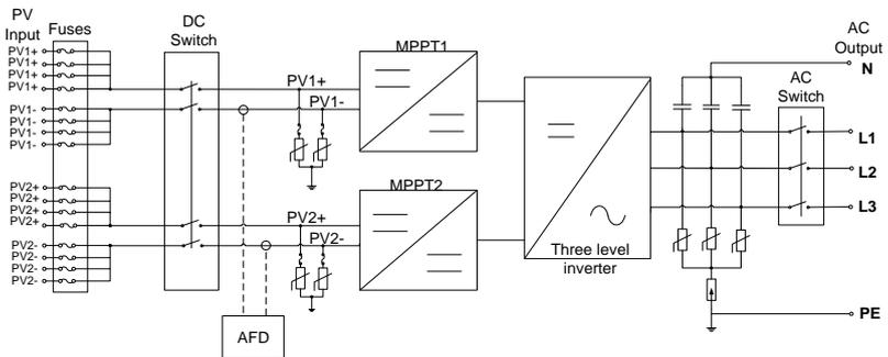
Figure 1.2 - Schematic Diagram of PVI 36TL Inverter
