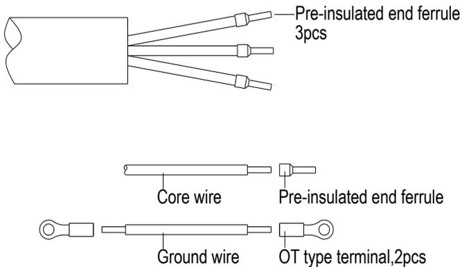
**Figure 2.31 - AC Output and Ground Cable Set Up**
