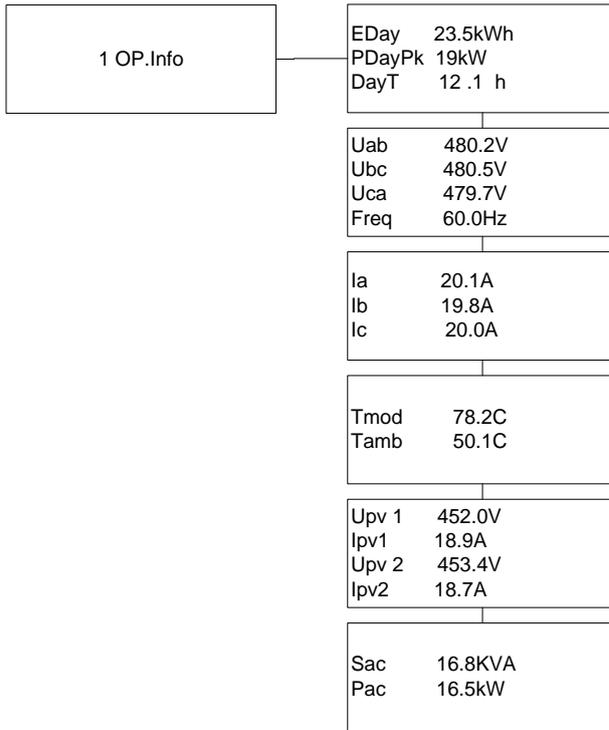
**Figure 4.8 - Operation information indication (PV independent mode)**
