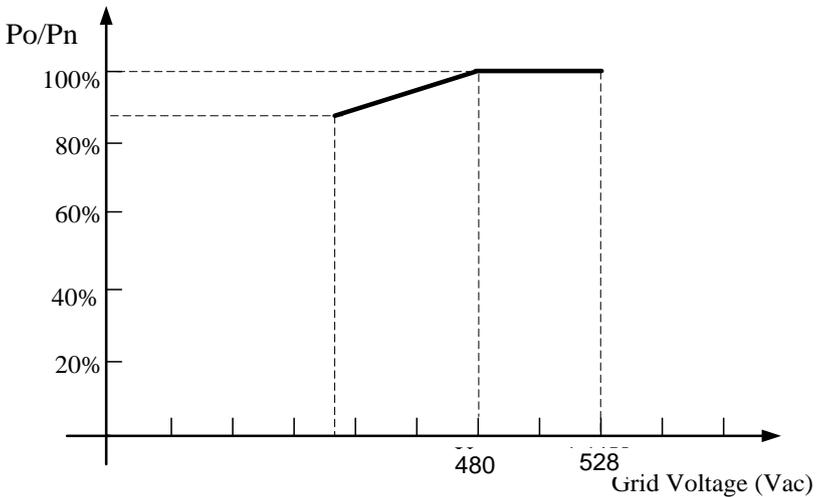
Figure 7.4 - PVI 36TL Derating Curve of Grid Voltage
