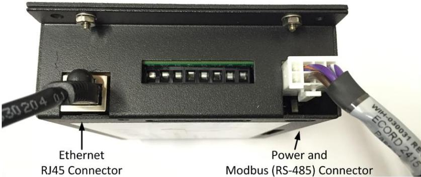
**Figure 2.39. - SolrenView Data Logger Connections.**
