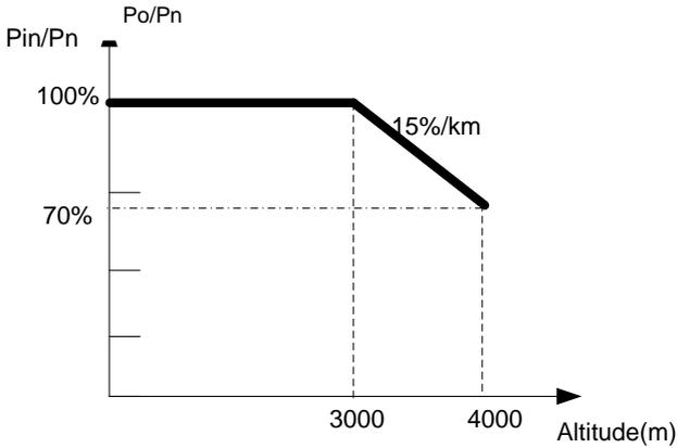
Figure 7.3 - PVI 36TL Derating Curve with High Altitude
