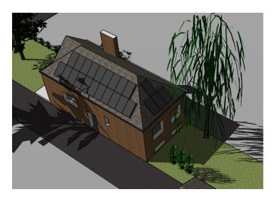
**Figure 5**: Shading pattern at 3PM. Large array partially shaded, small array entirely in the shadow.
